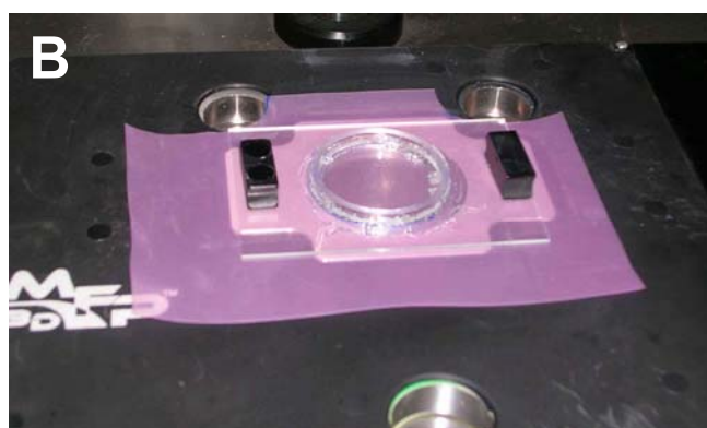
Plastic under sample offers more protection against fluid reaching bottom side of scanner.
