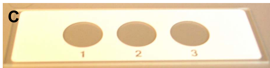
Plastic under sample offers more protection against fluid reaching bottom side of scanner.
