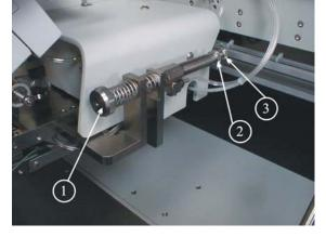
To adjust the low force setting, loosen the knurled lock nut  $\uparrow$  and turn the adjustment knob  $\rightarrow$  located behind the high force adjustment. When viewed from the rear of the bonder, counter-clockwise adjustments will reduce the bonding force. Use a gram gauge to measure the force.
