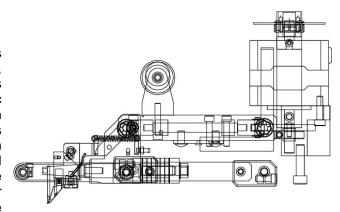
Clamps are air-opened and spring-closed, and have self-contained closure pivots. A separate pivot about an axis located to serve both overhead and angled feed generates the clamp motions along their lines of feed action.
