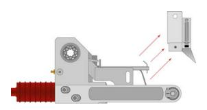
**2)** Holding the Tooling Head remove the clamp release screw and remove head assembly.
