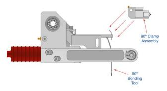
Insert the 90° Tooling head into the location the 45° was just removed from. Insert the Clamp Screw to secure Tooling Head. Align the clamp assembly so that the top surface of the clamps are flush with the top of the mounting surface. Tighten the Clamp Screw.
