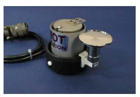
**-45C: Free Furnace Workholder:** for substrates up to 1.000" x 1.000", mechanical clamp, adjustable backstop with rotating die mirror presentation. Assembly No. 3800.009.
