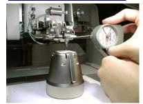
This option allows the operator to calibrate the "Force" setting by simply adjusting the force adjustment knob. This chrome plated knob  $\leftarrow$  is located directly to the right of the tooling head. To increase the bond force turn the knob counter-clockwise. To decrease the bond force turn the knob clockwise. Measure the force by placing a gram gauge just in front of the bond tool and lift until the machine beeps. Repeat to verify force is correct.
