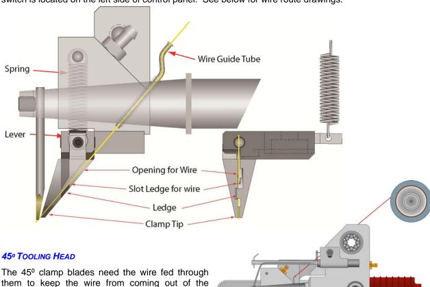
The 45° clamp blades need the wire fed through them to keep the wire from coming out of the clamps during looping. There is a small shelf that the wire needs to pass over before the tool is threaded.
