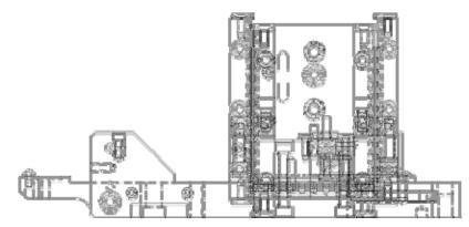
Dual counterweights balance the pantograph arm and the tool support individually, and they are complemented by an adjustable spring to counterbalance different tool assemblies. The resulting feel and balance are the best of all the model series.
